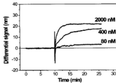
Three successive hybridization experiments with different 12-mer oligonucleotide concentrations using one array. *The concentration detection limit was calculated to be 10 nM.*
