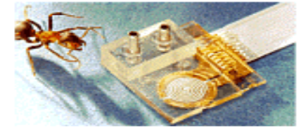
Micromembrane pump from the small series manufactured at the Research Center, as compared to the size of an ant.
