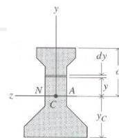
$$\sigma_{\max} = -\frac{E}{\rho} c \quad \text{farthest distance from N.A. to the surface}$$
