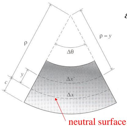
$$\begin{aligned}\varepsilon_x &= \frac{\delta}{L} = \frac{L_f - L_i}{L_i} \\ &= \frac{\Delta x' - \Delta x}{\Delta x} = \frac{(\rho - y)(\Delta\theta) - \rho(\Delta\theta)}{\rho(\Delta\theta)} \\ &= -\frac{1}{\rho} y\end{aligned}$$
