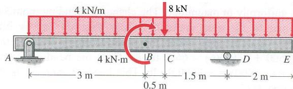
Find: ■ Write equations of  $V(x)$  and  $M(x)$  in the interval  $CD$
