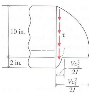
$$\begin{aligned} \tau &= \frac{VQ}{It} = \frac{V}{It} \int_{y_1}^c ty \, dy \\ &= \frac{V}{2I} (c_1^2 - y_1^2) = \frac{V}{2I} (8^2 - y_1^2) \quad \text{stem} \end{aligned}$$
