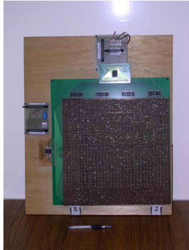
The equivalent 64x64-pixel PDP panel for driving emulation at CPT in 1999.
